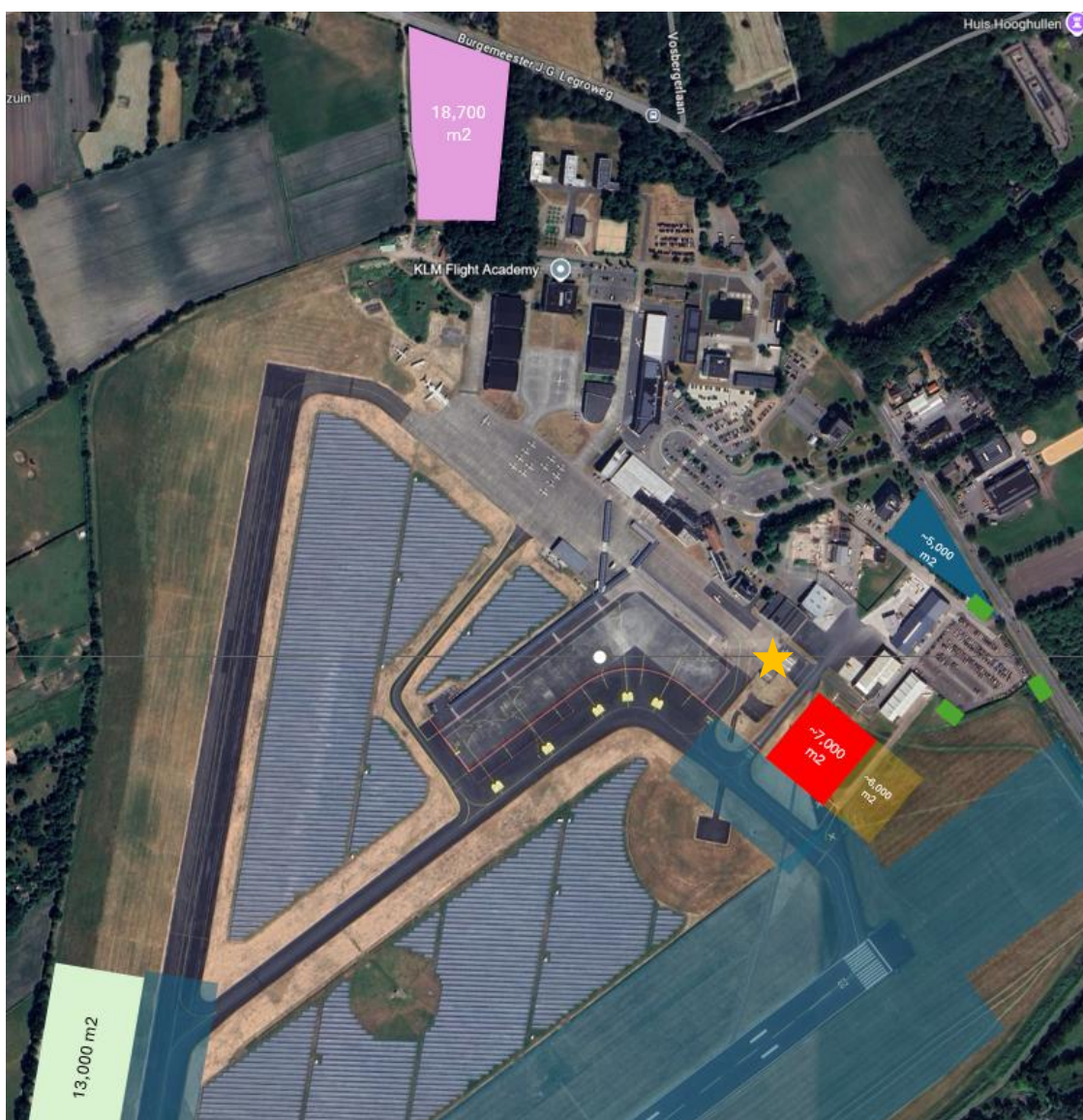
Figure 18: Initial Hydrogen Infrastructure Location (Red), Landside Refueling Station (Green), and Expansion Area (Orange). The star indicates the ATC tower.
